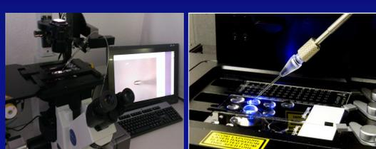
Semiautomated capillary device for aspiration of individual cells from cell suspensions (slides in the front) and deposition in individual cups (slides in the background)
